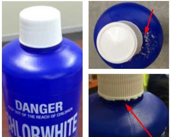
Above: One bottle as supplied new, and two showing leakage.
