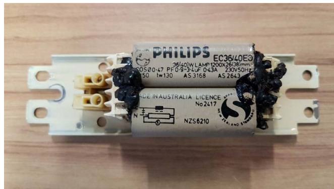
A burnt-out old-style wire-wound magnetic ballast from Christchurch Women's Hospital. The nominal service life is around 75,000 hours.
