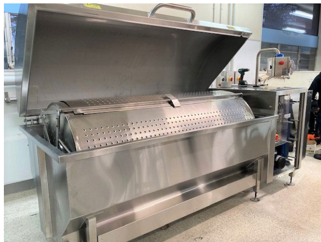
The new cook tank/tumble chiller
