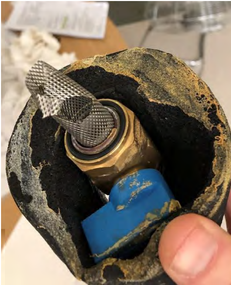
Image 1 – Failed drain valve
