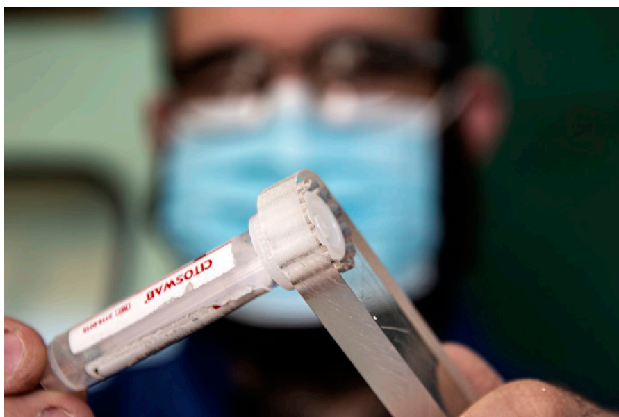
Uncapping a test tube using the decapping device
