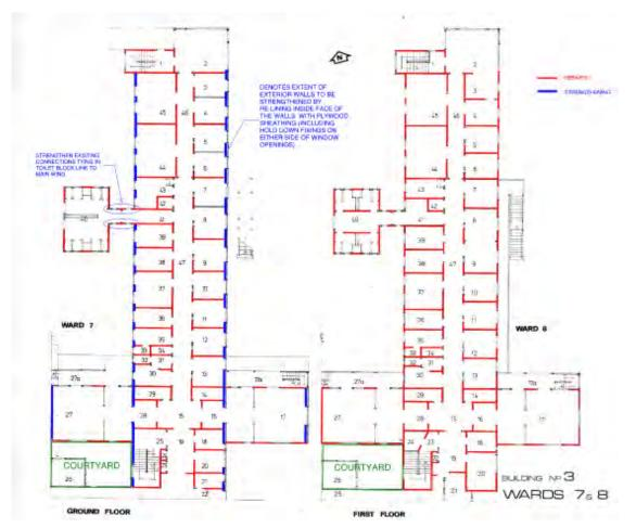
Figure 5-1: Ground Floor and First Floor Plan – Recommended Strengthening
