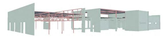
Figure 2-8: Image of NLTHA model used to analyse SOU Theatre (View from south-east)
