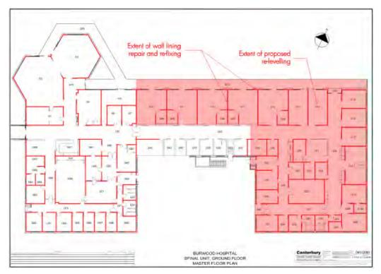
Figure 4-2: Ground Floor Plan - Damage Repairs
