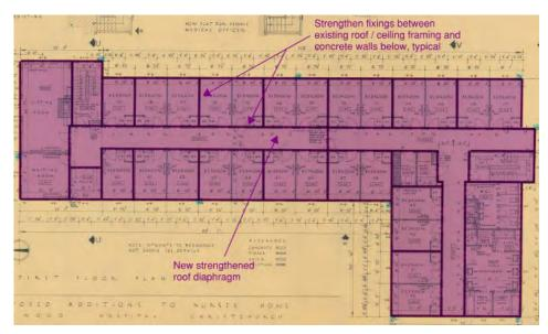
Figure 5-1: West Wing – First Floor Plan -Strengthening Recommended
