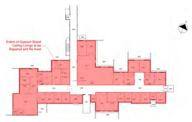
Figure 4-2: Reflected Ceiling Plan – Damage Repairs
