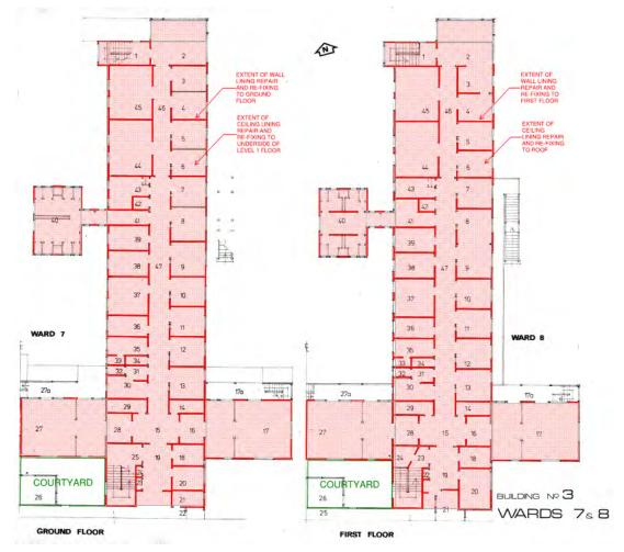
Figure 4-2: Ground and First Floor Plan - Damage Repairs
