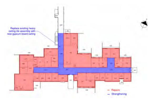
Figure 5-2: Ceiling Plan – Proposed Strengthening
