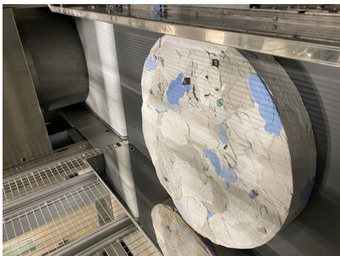
Water is squeezed rather than spun out of the clothes leaving them much drier
